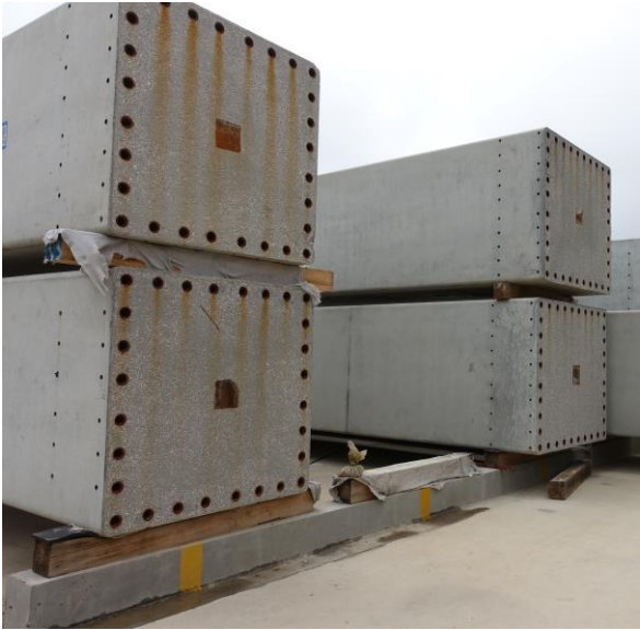
Figure 29 prefabricated element drilled part; connection prior to connection
