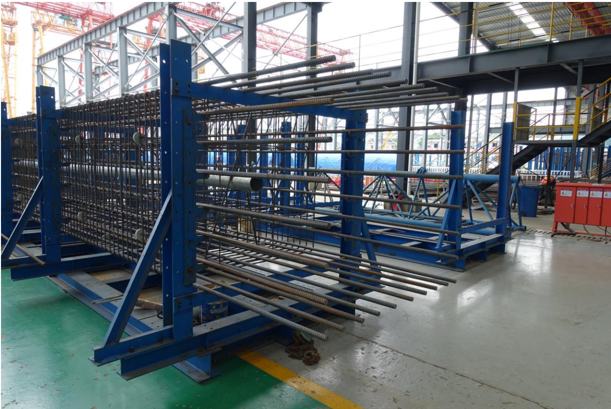
Figure 28: Reinforcement cage for prefabricated elements, to ensure the right position
